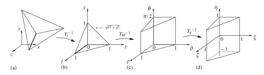
Figure 8. (a) Tetrahedron (Ω<sub>tet</sub>) with an edge on the singularity in the Cartesian (physical) coordinate (x, y, z) system; (b) tetrahedron (Â<sub>tet</sub>) in the volume coordinate (r̄, s̄, t̄) system; (c) transformed prism (Ω<sub>prism</sub>) in the mapped coordinate (ρ̄, θ̄, t̄') system; and (d) master prism (Â<sub>prism</sub>) in the master coordinate (ξ, η, ζ) system.
