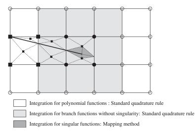
Figure 6. Numerical integration schemes with respect to enrichment functions.
