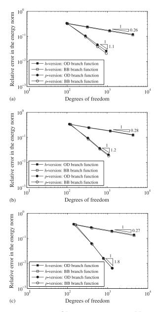
Figure 5. Comparison between the OD branch functions and the BB branch functions: (a) case I; (b) case II; and (c) case III.
