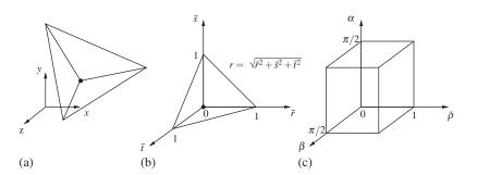
Figure 9. (a) Tetrahedron with a node on the singularity in the Cartesian (physical) coordinate (x, y, z) system; (b) tetrahedron in the volume coordinate  $(\bar{r}, \bar{s}, \bar{t})$  system; and (c) transformed hexahedron in the mapped coordinate  $(\bar{\rho}, \alpha, \beta)$  system.
