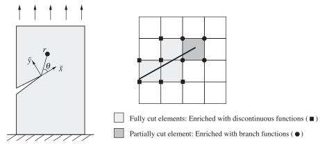
Figure 2. Enrichment cases with respect to the crack geometry.
