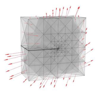
Figure 22. Edge-cracked panel with Mode I and Mode II boundary conditions from asymptotic expansion.
