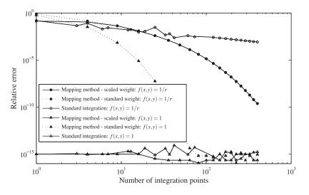
Figure 12. The effect of the scaled weight in the mapping method.
