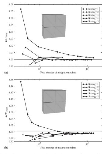
Figure 17. Normalized strain energy and stress intensity factor (SIF) for Strategies 1, 2, 3, 4 and 5 with respect to the sum of the total number of integration points used by all 24 elements: (a) normalized energy. Semi-log scale and (b) normalized SIF. Semi-log scale.
