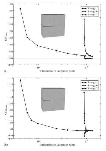
Figure 15. Normalized energy and stress intensity factor (SIF) for Strategies 1, 6 and 7. The horizontal axes show the sum of the number of quadrature points used by all 24 elements of the GFEM discretization: (a) normalized energy. Semi-log scale and (b) normalized SIF. Semi-log scale.
