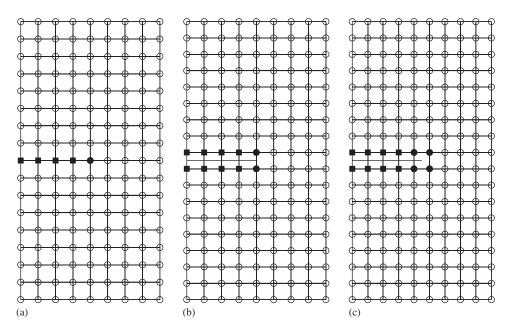
Figure 4. Finite element meshes for each case and local enrichment function types: (a) case I with the mesh grid of  $8 \times 16$ ; (b) case II with the mesh grid of  $8 \times 17$ ; and (c) case III with the mesh grid of  $9 \times 17$ .
