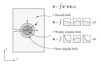
Figure 1. Example of singular behavior in linear elastic fracture mechanics problems. The notations are the following: **K** denotes the element stiffness matrix; **B** is the strain–displacement matrix; **D** indicates the constitutive matrix; *A* is the element area.
