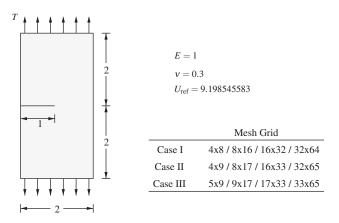
Figure 3. Geometry of problem and mesh grids for each case.
