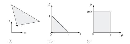
Figure 7. (a) Triangle with a node on the singularity in the Cartesian (physical) coordinate (x, y) system; (b) triangle in the area coordinate  $(\bar{r}, \bar{s})$  system; and (c) transformed rectangle in the mapped coordinate  $(\bar{\rho}, \bar{\theta})$  system.
