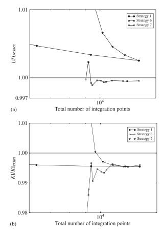
Figure 16. Zoom in of plots of Figures 15(a) and (b): (a) normalized energy. Semi-log scale and (b) normalized SIF. Semi-log scale.
