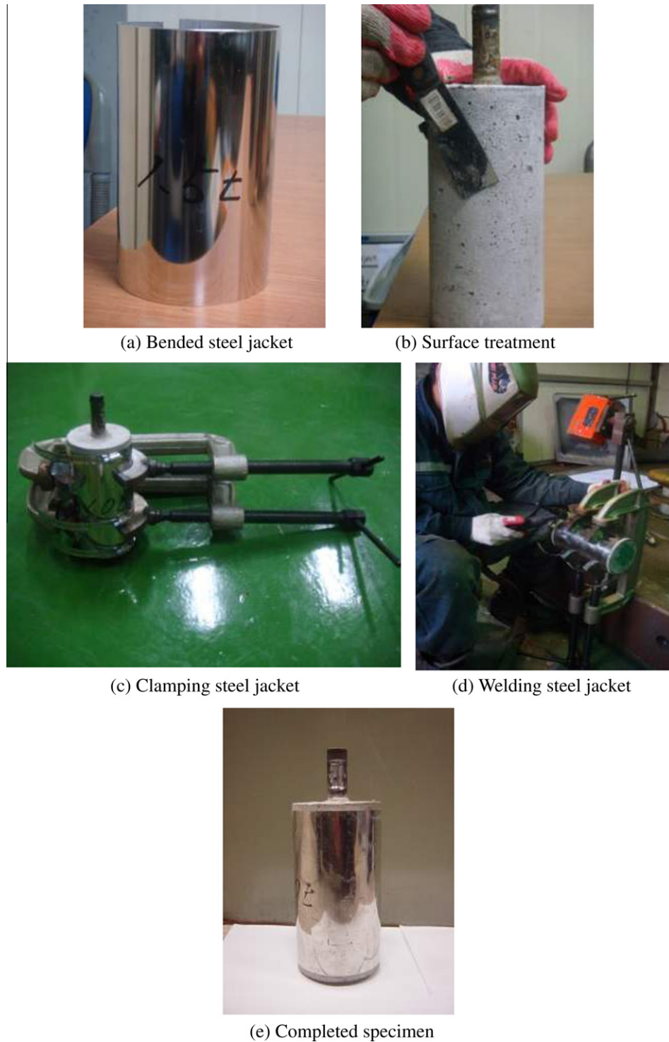
Fig. 1. Process for steel wrapping jackets.
