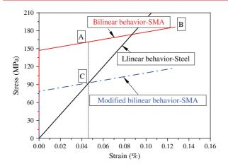
Figure 5. Bilinear behavior of the SMA wire.
