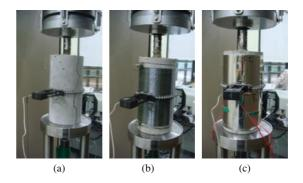
Figure 2. Specimen and test set-up for (a) plain concrete, (b) SMA wire jacket, and (c) steel plate jacket.
