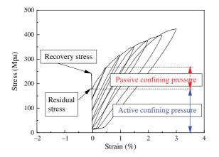
Figure 1. Cyclic tensile behavior of the SMA wire under residual stress.
