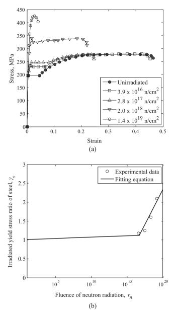
**Fig. 2.** (a) Uniaxial tension test results (Murty, 1984b) and (b) the yield strength ratio with respect to the fluence of neutron radiation.
