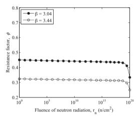
**Fig. 8.** Resistance factor for the target reliability indices,  $\beta$  = 3.04 and 3.44 considering compression-controlled failure data.
