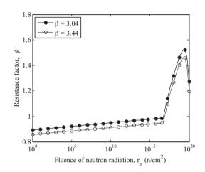
**Fig. 5.** Resistance factors for the target reliability indices,  $\beta$  = 3.04 and 3.44 considering tension-controlled failure data.
