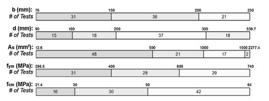
Fig. 4. The distributions of the values of design parameters.
