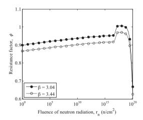
**Fig. 7.** Resistance factors for the target reliability indices,  $\beta$  = 3.04 and 3.44 considering the data in the transition range.
