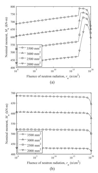
**Fig. 3.** Evaluation of the nominal moment (a) with the limited yielding stress, and (b) without limiting the yield stress.
