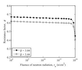
**Fig. 9.** Resistance factor for the target reliability indices,  $\beta$  = 3.04 and 3.44 considering compression-controlled data neglecting the uncertainties from the insufficient amount of data.
