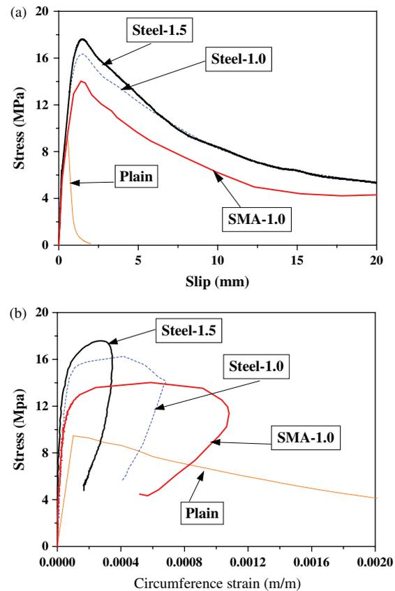
Figure 4. Relationships for (a) bond stress versus slip, and (b) bond stress versus circumferential strain.
