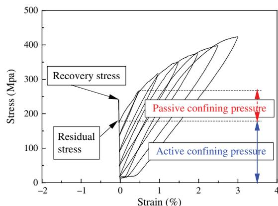
**Figure 1.** Cyclic tensile behavior of the SMA wire under residual stress.
