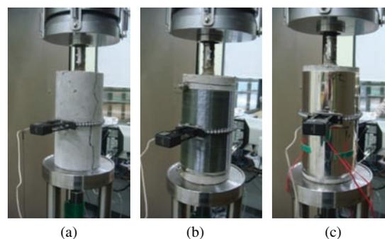
**Figure 2.** Specimen and test set-up for (a) plain concrete, (b) SMA wire jacket, and (c) steel plate jacket.
