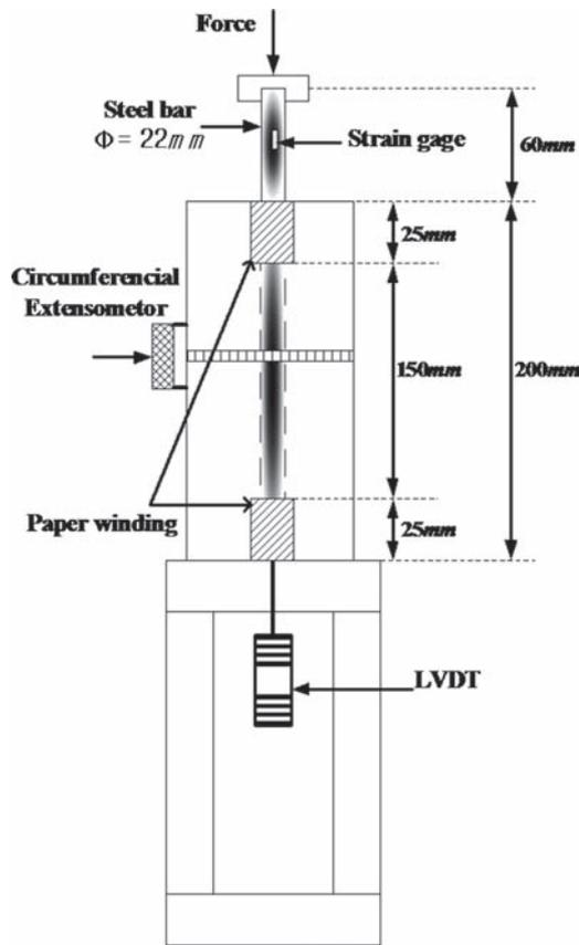
Figure 3. Schematics of test configuration.
